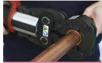
3. Complete the joint with the press tool
