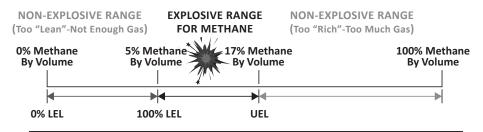
BELOW a specific LEL for a combustible gas, the air/gas mixture is too "lean" (not enough gas is present to burn). See the above visual diagram that applies to Methane only.
