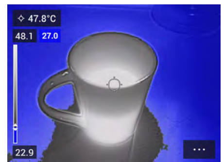
Below alarm : Highlights all pixels with a temperature below the specified temperature level.
