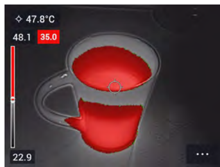
Above alarm : Highlights all pixels with a temperature above the specified temperature level.
