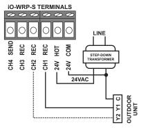
HEAT PUMP UPGRADE WITH ONLY TWO WIRES TO OUTDOOR UNIT
