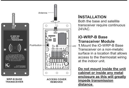
**2**. Once the base transceiver is mounted, take the access cover off by removing the two screws. Refer to the iO-WRP wiring diagram that best suits the application. Depending on the application, not all channels may be required.
