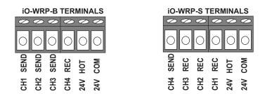
Please note the difference in terminal designations between the iO-WRP-B Base Module and the iO-WRP-S Satellite Module. The iO-WRP-B Base Module has three send and one receive channel. The iO-WRP-S Satellite Module has three receive and one send channel. SINGLE OR MULTI-STAGE COOLING WITH BROKEN WIRE TO OUTDOOR UNIT
