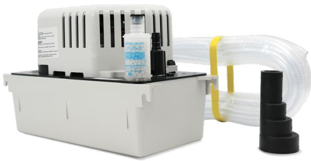
The Si-1801 centrifugal tank pump is capable of evacuating condensate at 132 gph with a 23' shut off head. It tolerates charged, high temperature and acidic condensates ( $\text{pH} > 2.5$ ) produced by gas condensing boilers.
