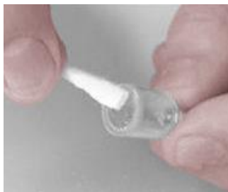
Figure 4. Cleaning Lamp Window
