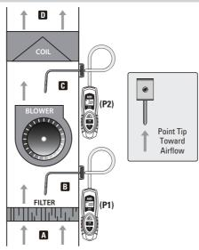
Static pressure testing ensures if the equipment is operating within factory specifications.
