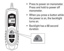
Note: The Manometer has a 10 second count down upon powering on.
