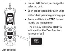
Note: Prior to testing, the Manometer must be zeroed. Do this in a non pressurized area with no hoses connected.
