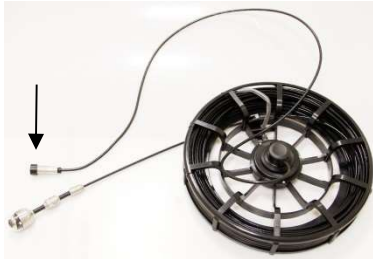
Fig. 76: Viper removed from the case, monitor plug covered by a lid
